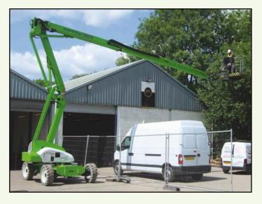
The **HR21 Hybrid AWD** also incorporates Niftylift's new **ToughCage** technology. Its tough impact resistant composite base and larger cross-section steel cage give extra strength and durability, both protecting the operator and reducing the risk of damage to the cage.
